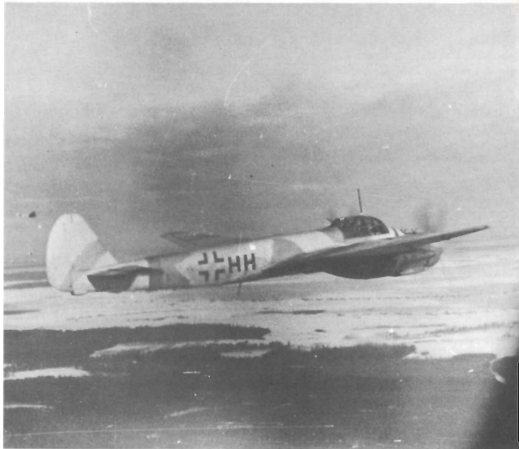
16 A Junkers Ju88C-6 of NJG 100, the only night fighter unit to use the type on the Eastern Front. The aircraft is in an unusual three-tone camouflage scheme, with the swastika overpainted and a yellow band around the rear fuselage. The lower fin has the fairing for the aerials of tail warning radar, but the aerial itself does not appear to be fitted.
