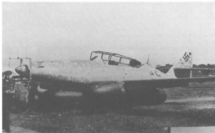
41. 'Red 12' of NJG 11, an Me262B-1a/U1 W. Nr 111980 with black underside paintwork and mottled blue-grey camouflage on top, seen on a Berlin airfield after the war. (Via EJC)
